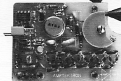
Model A-101 mounted on the MD-501 AmpTektron ® , complete with CEM, high voltage power supply and line driver.
