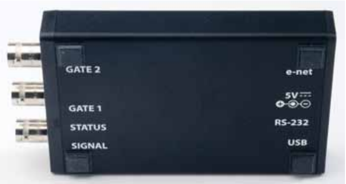
Figure 4. MCA8000D Back View
